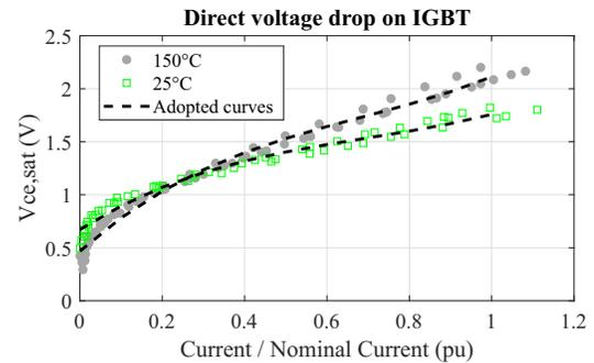
FIGURE 22. Voltage drop across silicon IGBTs. Behavior modeled by a third-degree equation, obtaining a determination coefficient ( $R^2$ ) of 0.9771 for 25 °C and 0.9865 for 150 °C.
