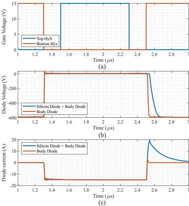
**FIGURE 11. Diode's behavior: (a) gate voltage of the power transistors. (b) Diodes voltage drop. (c) Diodes current flow. Conditions:  $I_{load} = 15\text{ A}$  and  $T_{vj} = 150\text{ }^{\circ}\text{C}$ . Results were obtained using LTspice software.**
