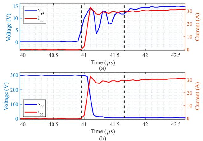
FIGURE 15. Experimental turn-on transient for IGBT: (a)  $v_{ce}$  and  $i_{ce}$  and (b)  $v_{ge}$  and  $i_{ce}$ . Conditions:  $I_{load} = 30\text{ A}$  and  $V_{DC} = 300\text{ V}$ .
