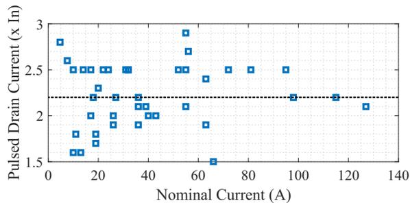
FIGURE 24. Pulsed current data for 1200 V MOSFETs with average value highlighted.
