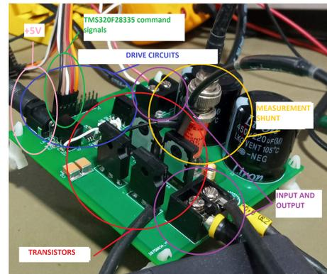
**FIGURE 13. Double-pulse test setup built.**
