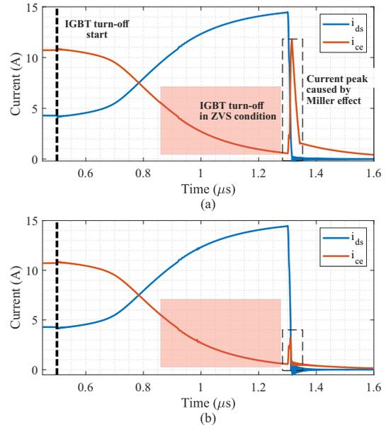
FIGURE 8. Simulation of the HyS turn-off transient composed of a 15 A Si-IGBT and a 13 A SiC-MOSFET. (a) Implementation without the Miller clamp; (b) Implementation with Miller clamp. Conditions:  $I_{load} = 15$  A and  $T_{vj} = 150$  °C. Results were obtained using LTspice software.
