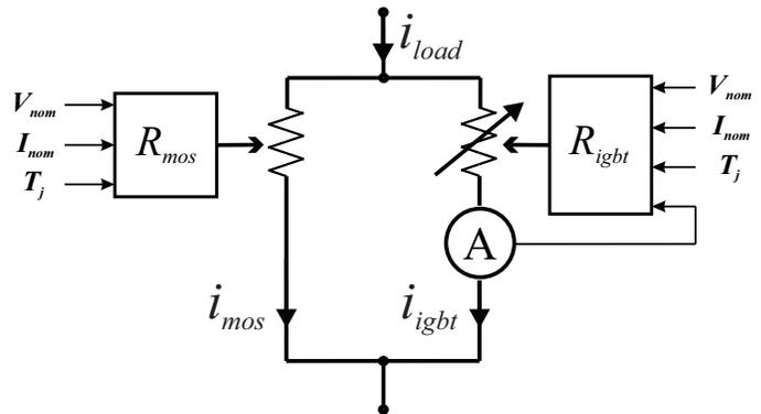
FIGURE 5. Current sharing modeling during the conduction period.
