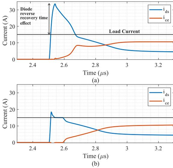
FIGURE 9. Simulation of the HyS turn-on transient composed of a 15 A Si-IGBT and a 13 A SiC-MOSFET. (a) Implementation using IGBT with diode; (b) Implementation employing diodeless IGBT. Conditions:  $I_{load} = 15$  A and  $T_{vj} = 150$  °C. Results were obtained using LTspice software.
