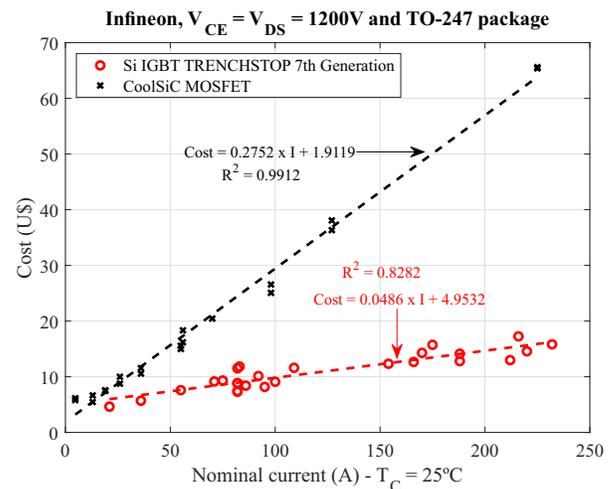
FIGURE 1. Unit cost comparison of Si-IGBT and SiC-MOSFET from Infineon Technologies company. Devices with 1200V blocking voltage and TO-247 package [5]. Data collected in May 2024.
