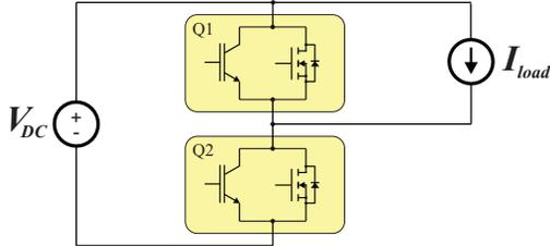
FIGURE 7. Schematic of the DPT with two HyS.
