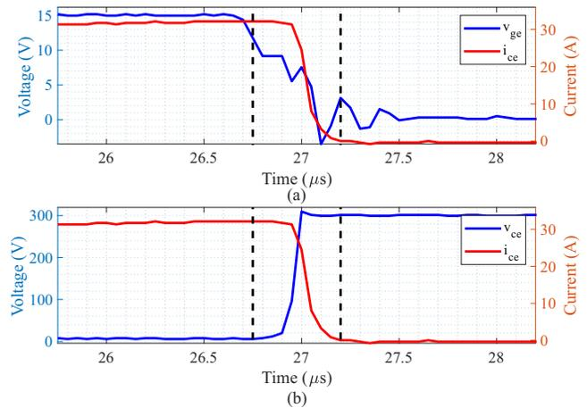
FIGURE 14. Experimental turn-off transient for IGBT: (a)  $v_{ce}$  and  $i_{ce}$  and (b)  $v_{ge}$  and  $i_{ce}$ . Conditions:  $I_{load} = 30\text{ A}$  and  $V_{DC} = 300\text{ V}$ .
