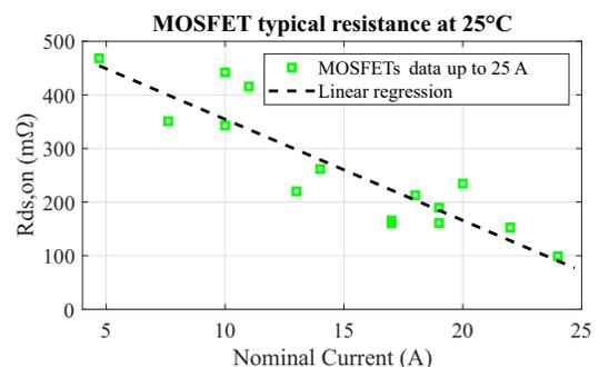
FIGURE 20.  $R_{ds}$  typical data as a function of 1200 V MOSFETs' rated currents up to 25 A. Affine function with determination coefficient ( $R^2$ ) of 0.9438.
