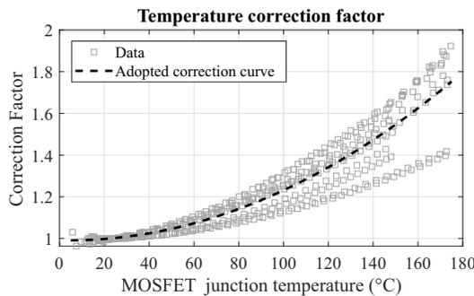
FIGURE 21. SiC-MOSFET conduction resistance correction factor as a function of junction temperature. Adopted curve whose determination coefficient ( $R^2$ ) was 0.8617.
