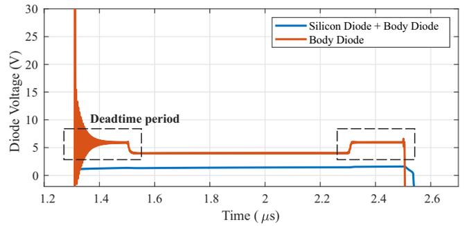
**FIGURE 12. Zoomed view of Fig. 11 b. highlighting the deadtime period and diode voltage drop across the hybrid pair for the IGBT with and without FWD.**
