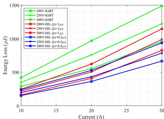
FIGURE 19. Comparison of losses among circuits featuring IGBTs, HyS with  $0.5 \mu\text{s}$  delay, and HyS with  $1 \mu\text{s}$  delay. Results are provided for three levels of DC voltage and three circuit current values.
