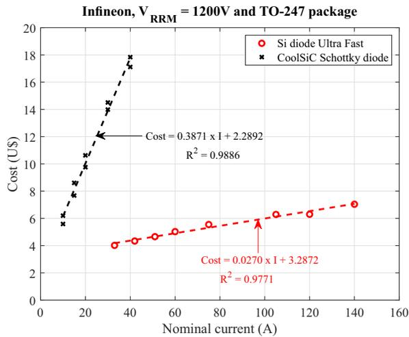
FIGURE 2. Unit cost comparison of Si diodes and SiC Schottky diodes from Infineon Technologies company. Devices with 1200V blocking voltage and TO-247 package [5]. Data collected in May 2024.
