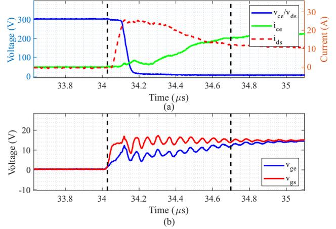
FIGURE 17. Experimental turn-on transient for HyS with a  $0.5 \mu\text{s}$  turn-on delay: (a) voltage drop and current sharing and (b) gate voltages. Conditions:  $I_{load} = 30 \text{ A}$  and  $V_{DC} = 300 \text{ V}$ .
