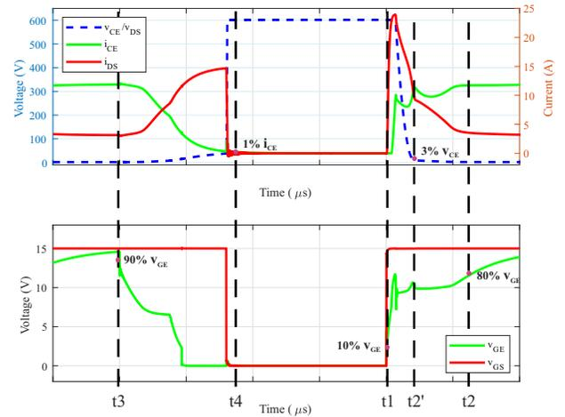
FIGURE 10. Example of integration period determination to calculate the energies for Si-IGBT and SiC-MOSFET in a HyS.
