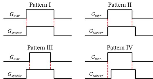
FIGURE 4. Hybrid Switch gate signals patterns investigated in the literature.
