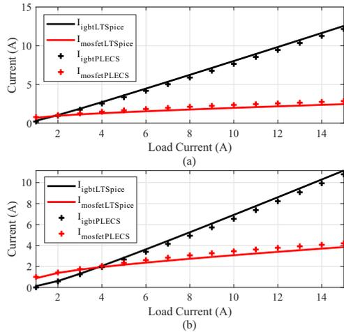
FIGURE 23. Current division in spice models and models obtained for the pair comparison: (a) MOSFET 4.7 A and IGBT 15 A and (b) MOSFET 13 A and IGBT 15 A.
