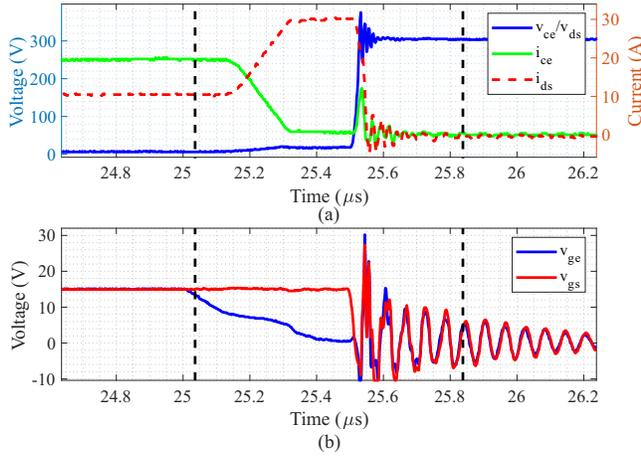
FIGURE 16. Experimental turn-off transient for HyS with a  $0.5 \mu\text{s}$  turn-off delay: (a) voltage drop and current sharing, and (b) gate voltages. Conditions:  $I_{load} = 30 \text{ A}$  and  $V_{DC} = 300 \text{ V}$ .
