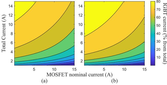
FIGURE 6. Percentage of the total circuit current flowing through the IGBT during the conduction period with a nominal current of (a) 15 A and (b) 25 A. Condition:  $T_{vj} = 150$  °C. Results were obtained using PLECS software.
