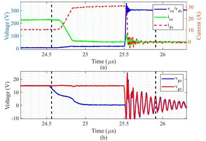
FIGURE 18. Experimental turn-off transient for HyS with a  $1 \mu\text{s}$  turn-off delay: (a) voltage drop and current sharing and (b) gate voltages. Conditions:  $I_{load} = 30 \text{ A}$  and  $V_{DC} = 300 \text{ V}$ .
