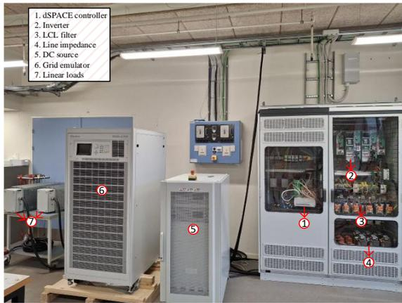
FIGURE 13. Lab setup for obtaining experimental results.
