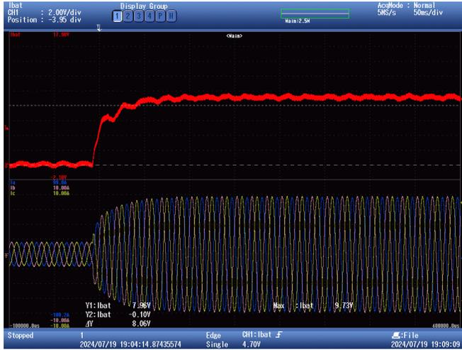
FIGURE 11. Battery current response for reference tracking.
