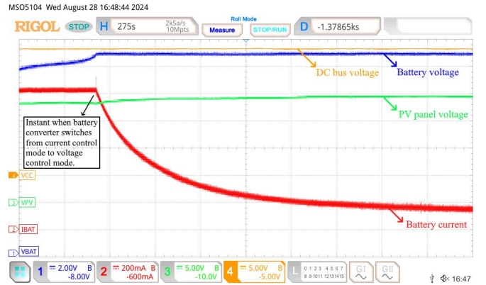
FIGURE 10. Battery charging by CC-CV method: curves of DC bus voltage, PV panel voltage, battery voltage and current.
