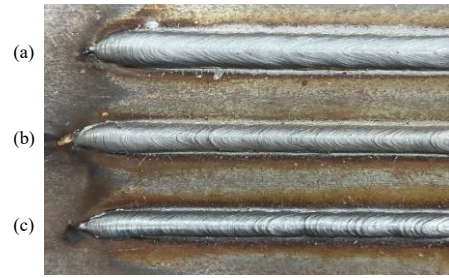
FIGURE 18. Welding using a prototype with different set-points: (a) 18 V – 5.0 m/min, (b) 16 V – 4.5 m/min, and (c) 14 V – 3.5
