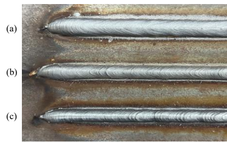
FIGURE 18. Welding using a prototype with different set-points: (a) 18 V – 5.0 m/min, (b) 16 V – 4.5 m/min, and (c) 14 V – 3.5
