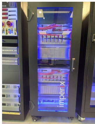
FIGURE 4. Experimental platform used for control tests, composed of: converters, sensing and signal conditioning boards, Imperix B-Box RCP connected to a computer.
