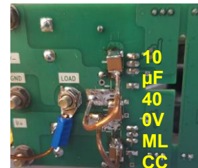
FIGURE 9. Arrangement for drain current measurements.
