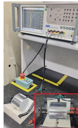
FIGURE 14. Equivalent series resistance measurement of the capacitive element.
