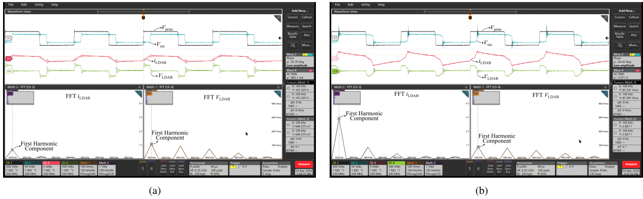
FIGURE 8. Experimental waveforms for first harmonic approximation: (a) CH1 - V_{prim} ; CH2 - V_{sec} ; CH3 - i_{LDAB} ; CH4 - V_{LDAB} . i_{bias} = 0 ; (b) i_{bias} = 1 A.
