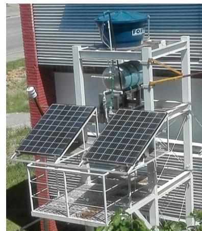
Fig. 6. Experimental setup of the two KC200 PV modules.
