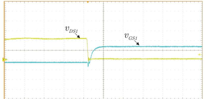
Fig. 15. Experimental waveforms of Full-Bridge ZVS-PWM S-PPC converter for  $V_{in} = 64$  V. Scales - time:  $1 \mu\text{s}/\text{div}$ ; switch  $S_1$  drain-source voltage ( $v_{DS1}$ ):  $30 \text{ V}/\text{div}$ ; switch  $S_1$  gate-source voltage ( $v_{GS1}$ ):  $10 \text{ V}/\text{div}$ .
