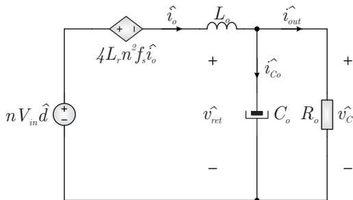
Fig. 8. Small-signal modeling of Full-Bridge ZVS-PWM.
