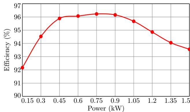
Fig. 18. Experimental efficiency of Full-Bridge ZVS-PWM S-PPC converter.
