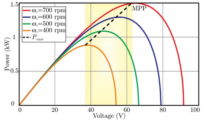
Fig. 6. Electrical power curves ( $P_{in}$ ) as a function of the S-PPC input voltage ( $V_{in}$ ) for angular speeds from 400 to 700 rpm.
