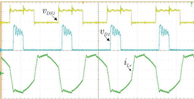
Fig. 13. Experimental waveforms of Full-Bridge ZVS-PWM S-PPC converter for  $V_{in} = 64$  V. Scales - time:  $10 \mu\text{s}/\text{div}$ ; switch  $S_1$  drain-source voltage ( $v_{DS1}$ ):  $50 \text{ V}/\text{div}$ ; diode  $D_1$  block voltage ( $v_{D1}$ ):  $200 \text{ V}/\text{div}$ ; resonant current ( $i_{LR}$ ):  $20 \text{ A}/\text{div}$ .
