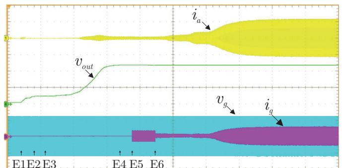
Fig. 16. Experimental waveforms of the proposed system startup connected in the grid. Scales - time:  $20 \text{ s}/\text{div}$ ; PMSG phase current ( $i_a$ ):  $20 \text{ A}/\text{div}$ ; dc bus voltage ( $v_{out}$ ):  $100 \text{ V}/\text{div}$ ; grid voltage ( $v_g$ ):  $100 \text{ V}/\text{div}$ ; grid current ( $i_g$ ):  $20 \text{ A}/\text{div}$ .
