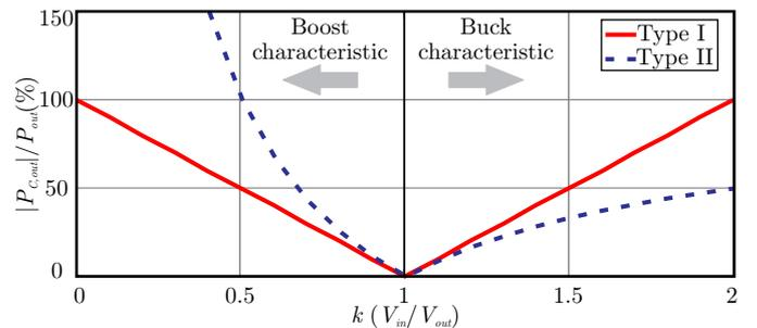
Fig. 4. Active power in S-PPC type I and type II plotted in function of parameter  $k$ .
