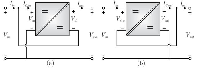
Fig. 3. S-PPC connections schemes. (a) Input-parallel-output-series (Type I). (b) Input-series-output-parallel (Type II).
