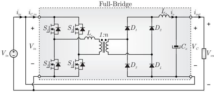
Fig. 7. Full-Bridge ZVS-PWM topology connected as S-PPC in input-parallel-output-series configuration.
