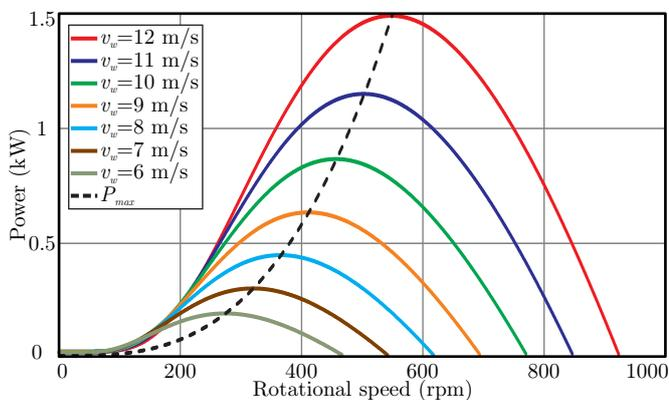
Fig. 5. Curves of mechanical power in function of angular rotational speed  $P_{mec}(\omega_r)$  for wind speeds from 6 to 12 m/s.
