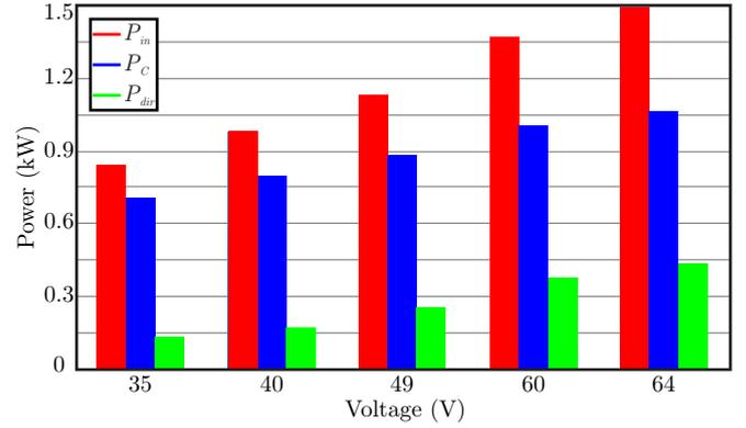
Fig. 9. Input power ( $P_{in}$ ), active power processed ( $P_C$ ), and direct power flow ( $P_{dir}$ ) in Full-Bridge ZVS-PWM S-PPC for different operational points of SWT system.
