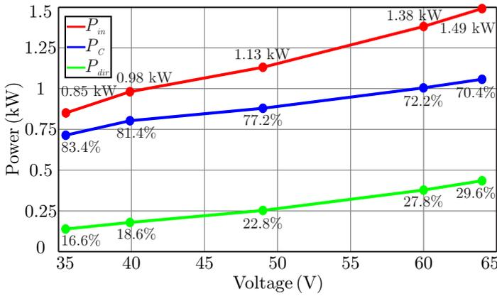
Fig. 17. Experimental curves of input power ( $P_m$ ), processed power ( $P_c$ ), and direct power ( $P_{dir}$ ) in Full-Bridge ZVS-PWM S-PPC for different input voltages.
