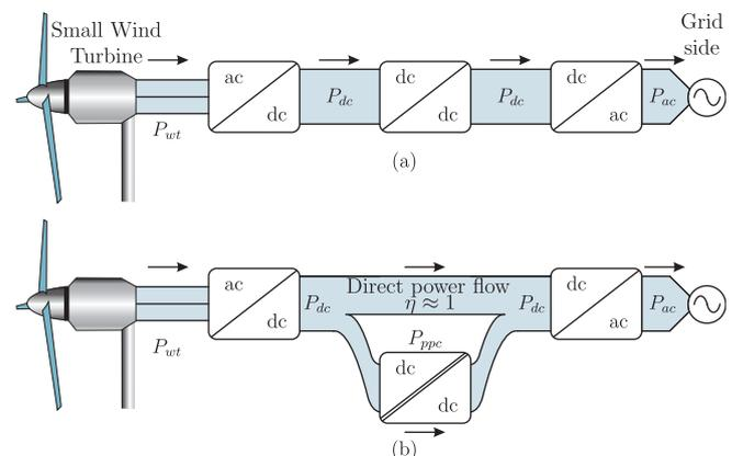
Fig. 1. Power flow of a three-stage SWT processing system employing a: (a) FPC and (b) PPC.
