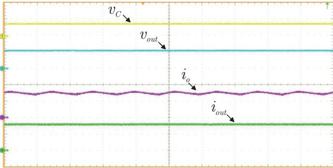
Fig. 12. Experimental waveforms of Full-Bridge ZVS-PWM S-PPC converter for  $V_{in} = 64$  V. Scales - time:  $10 \mu\text{s}/\text{div}$ ; converter output voltage ( $v_C$ ):  $200 \text{ V}/\text{div}$ ; dc bus voltage ( $v_{out}$ ):  $200 \text{ V}/\text{div}$ ; converter output current ( $i_o$ ):  $4 \text{ A}/\text{div}$ ; dc bus current ( $i_{out}$ ):  $4 \text{ A}/\text{div}$ .
