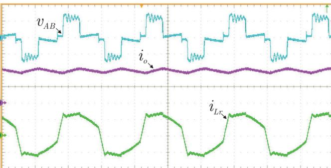
Fig. 14. Experimental waveforms of Full-Bridge ZVS-PWM S-PPC converter for  $V_{in} = 64$  V. Scales - time:  $10 \mu\text{s}/\text{div}$ ; transformer primary side voltage ( $v_{AB}$ ):  $50 \text{ V}/\text{div}$ ; converter output current ( $i_o$ ):  $3 \text{ A}/\text{div}$ ; resonant current ( $i_{LR}$ ):  $30 \text{ A}/\text{div}$ .
