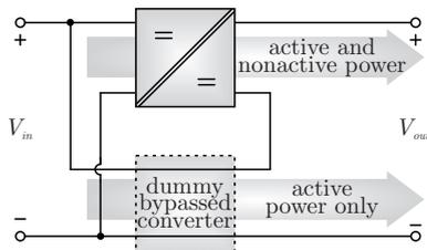
Fig. 2. Active and nonactive power processing on S-PPCs.
