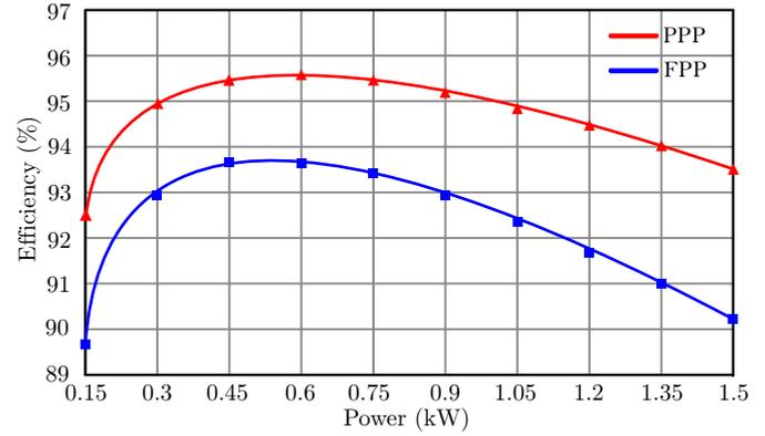
Fig. 19. Simulated efficiency of partial-power processing (PPP) and full-power processing (FPP).
