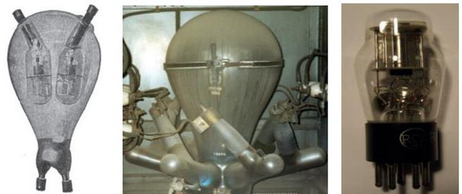
Fig. 1. Mercury Arc Valve (Rectifier): The original prototype by P. C. Hewitt in 1902 (left) and an old industry product (center) and a more recent RC85 thyatron [7, 8].
