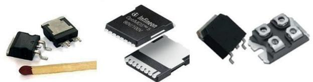
Fig. 6. MOSFETs for low- to medium-power applications.
