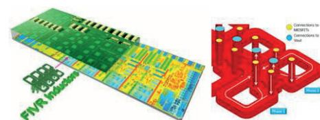
Fig. 12. Board integration of inductors (left and center) and switched-capacitor circuit (right) [36, 37].
