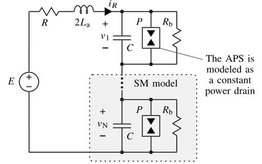
Fig. 3. Equivalent phase circuit during the *Uncontrolled and active* precharge stage.
