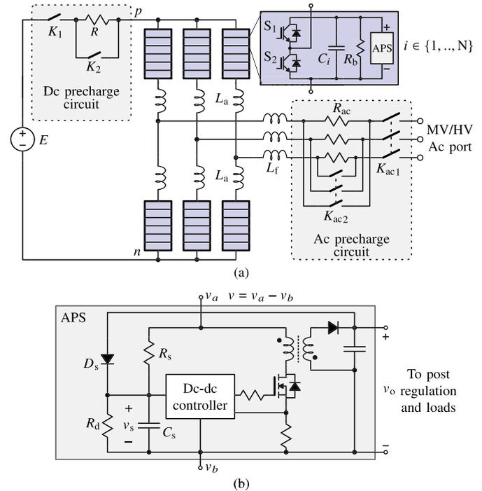
Fig. 1. (a) MMC converter and its ac and DC precharge circuits (adapted from [7]). (b) Simplified circuit of an APS based on a flyback converter.
