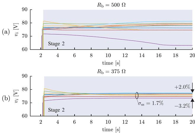
Fig. 12. Capacitor voltages during precharge for (a)  $R_b = 500 \Omega$  ( $\hat{V}_b = 0.963$ ,  $\gamma = 1.09$ ) and (b)  $R_b = 375 \Omega$  ( $\hat{V}_b = 0.96$ ,  $\gamma = 1.43$ ).
