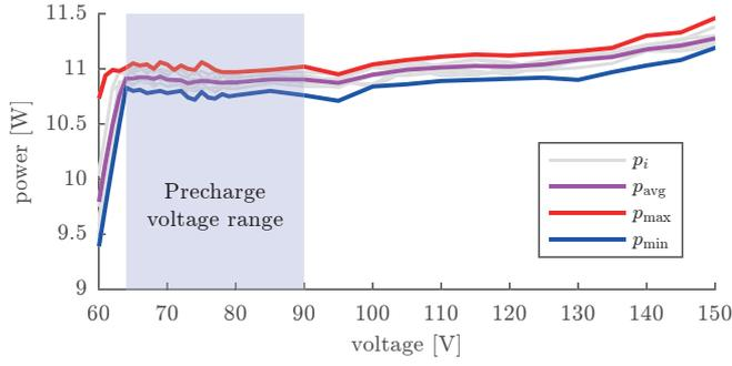
Fig. 2. Power consumption  $p_i$ , for  $i \in \{1, \dots, 10\}$ , of the APSs used in this work as a function of SM capacitor voltage  $v$ . Average, maximum and minimum values are also shown.
