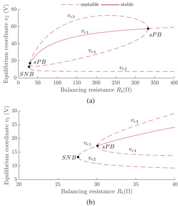
Fig. 4. Bifurcation diagram of (6) for  $R_b$  as the varying parameter in the range  $[0, 400]\Omega$  (for  $E = 150V$ ,  $R = 100\Omega$  and  $P = 10W$ ). Full bifurcation diagram (a) and zoom around the saddle-node bifurcation (b).
