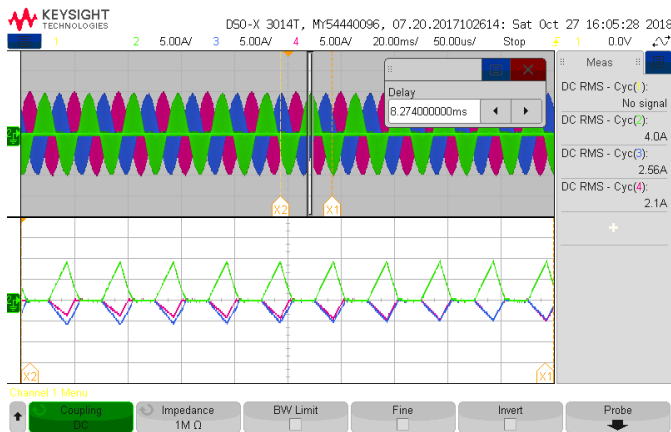
Fig. 9. Waveforms of the currents i_{r1} (blue), i_{s1} (red), i_{t1} (green) for 60Hz input frequency and the detail of the waveforms when the maximum value of i_{t1} occurs.
