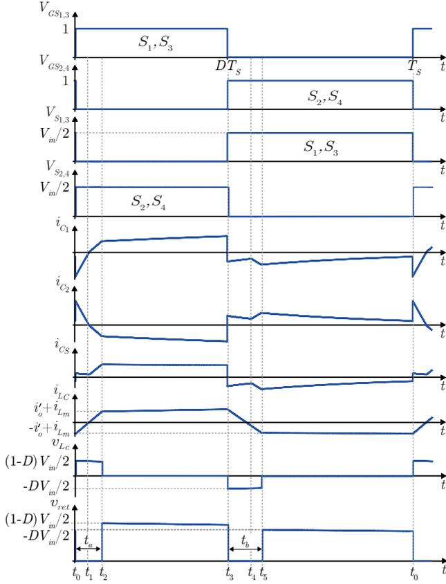
Fig. 3. Typical waveforms of the proposed converter.
