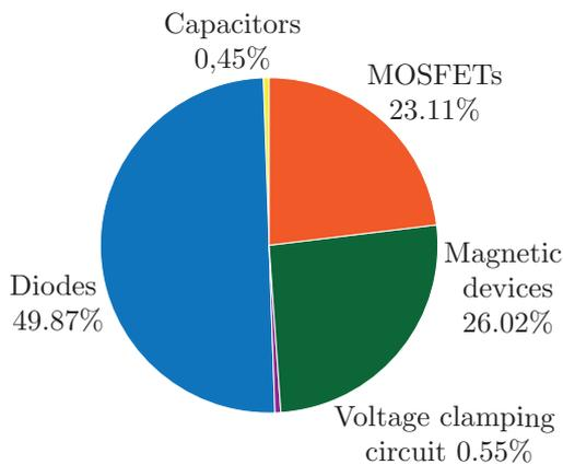
Fig. 19. Theoretical distribution of losses in the converter power stage.
