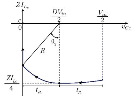
Fig. 9. State plane trajectory for the resonant stage of soft commutation.
