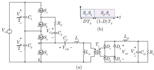
Fig. 1. (a) DC-DC hybrid half-bridge converter. (b) Gate signals.
