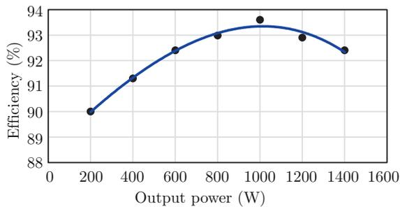
Fig. 18. Efficiency of the experimental prototype of the proposed converter.
