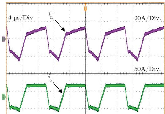
Fig. 13. Current waveforms in the transformer primary and secondary windings.
