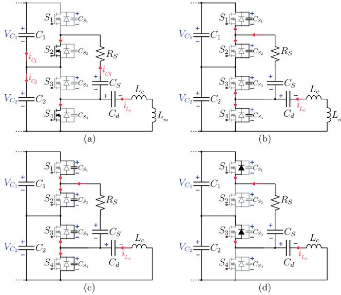
Fig. 7. Topological stages during commutation. (a) Before  $S_2$  and  $S_4$  turn off ( $t_0 - t_6$ ). (b) Linear stage ( $t_0 - t_{0a}$ ). (c) Resonant stage ( $t_{0a} - t_{0b}$ ). (d) End of commutation ( $t_{0b} - t_{0c}$ ).
