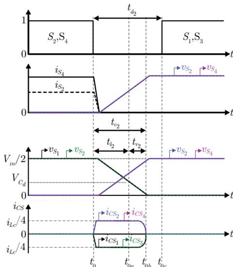
Fig. 8. Typical waveforms for the commutation initiated at time  $t = t_6$ .
