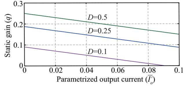
Fig. 4. Static gain of the proposed converter as a function of  $\bar{I}'_o$  for different values of the duty cycle  $D$ .
