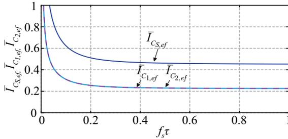
Fig. 6. Graphic representation of effective values of the currents in  $C_1$ ,  $C_2$  and  $C_S$ , normalized in relation to  $I'_o$  as a function of  $f_s \tau$ , for  $D = 0.45$ .
