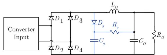
Fig. 12. Voltage clamping circuit to limit the voltage across diodes  $D_1$ ,  $D_2$ ,  $D_3$  and  $D_4$ , included in the experimental prototype.
