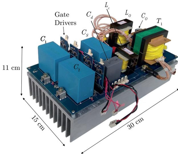
Fig. 10. Experimental prototype of the ZVS-PWM-SC asymmetrical half- bridge dc-dc converter.
