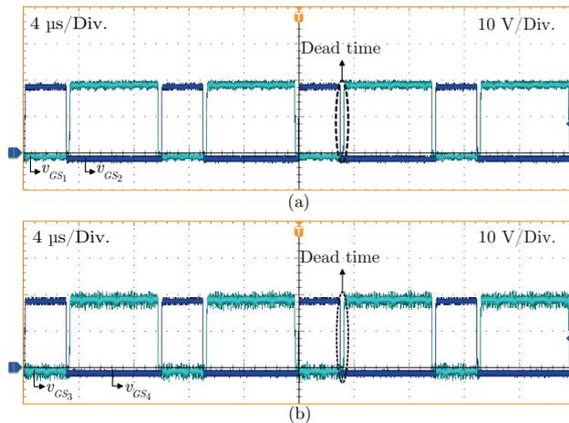
Fig. 11. (a) Gate signals of  $S_1$  and  $S_2$ . (b) Gate signals of  $S_3$  and  $S_4$ .
