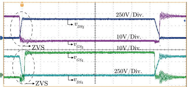
Fig. 16. Gate signals and voltage stress of semiconductors  $S_3$  and  $S_4$ .
