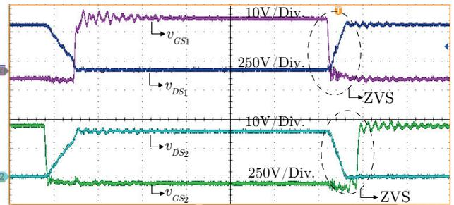
Fig. 15. Gate signals and voltage stress of semiconductors  $S_1$  and  $S_2$ .
