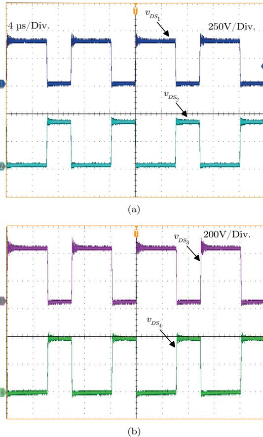
Fig. 14. (a) Voltages across semiconductors  $S_1$  and  $S_2$ . (b) Voltages across semiconductors  $S_3$  and  $S_4$ .
