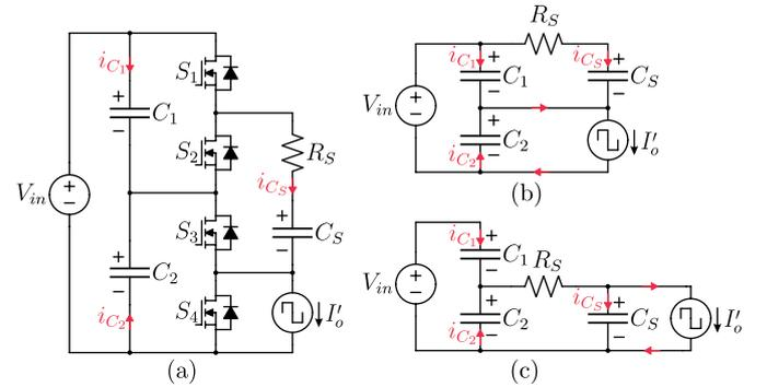
Fig. 5. (a) Simplified representation of the converter. (b) Equivalent circuit for the first stage of operation. (c) Equivalent circuit for the second stage of operation.
