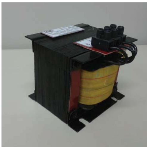
Fig. 14. Photograph of the Scott autotransformer. Dimensions are 115mm x 70mm x 94mm.
