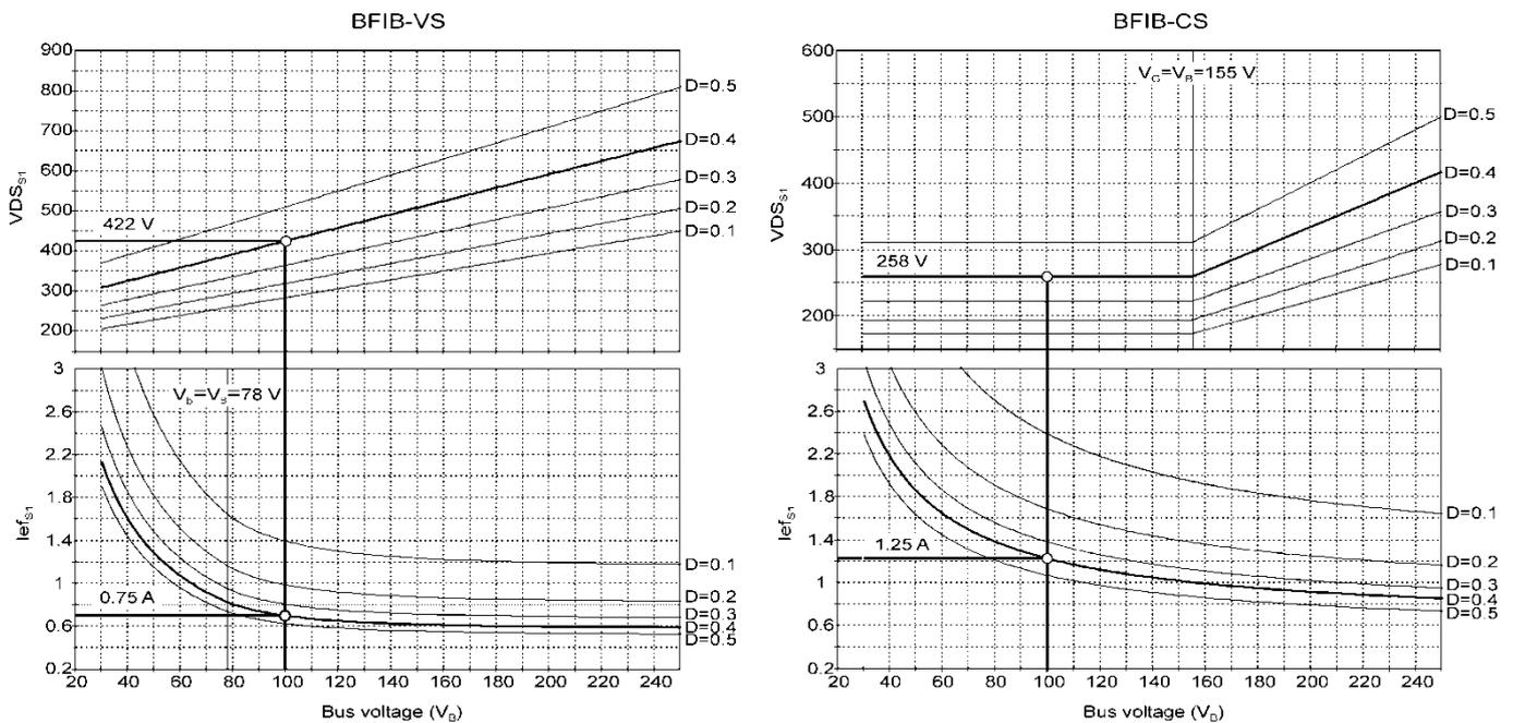
Fig. 8. Defined shared switch drain-to-source voltage and rms current to  $V_B=100$  V and  $D=0.4$ .
