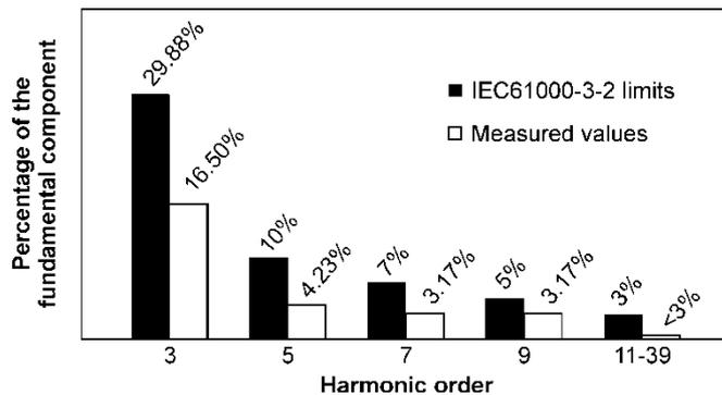
Fig. 11. Measured input current harmonics compared to the IEC61000-3-2 standard limits for the BFIB-VS.
