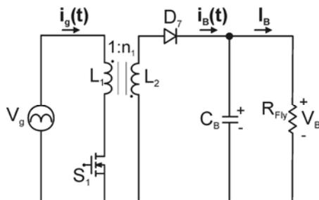
Fig. 4. PFC stage equivalent circuit.
