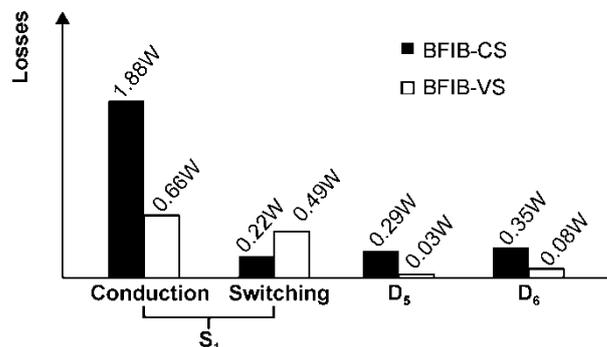
Fig. 12. Comparison between losses in the two electronic ballasts configurations.
