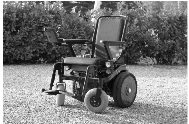
Fig. 1. Electric wheelchair equipped with proposed wheel motor drive prototypes.
