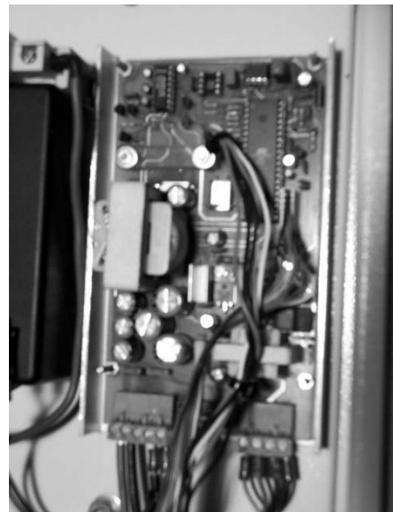
Fig. 20 – Picture of the charge controller in operation.
