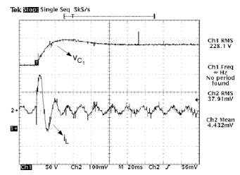
Fig. 9. Voltage on DC bus capacitor  $C_1$  and line current (10mV/A).
