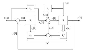
Fig. 1. Basic state feedback control structure.
