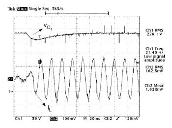
Fig. 10. Voltage on DC bus capacitor  $C_1$  and line current (10mV/A).
