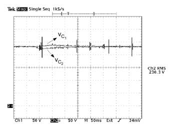
Fig. 12. Voltage on DC bus capacitor banks  $C_1$  and  $C_2$ .
