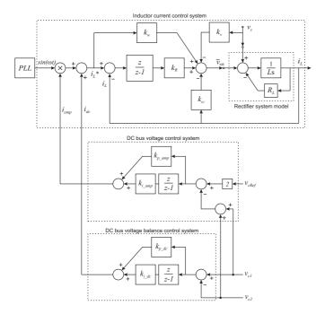
Fig. 3. Rectifier control system diagram.
