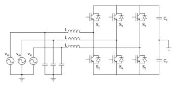
Fig. 2. Three-phase rectifier schematic diagram.
