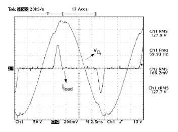
Fig. 16. Output voltage and load current (10mV/A).
