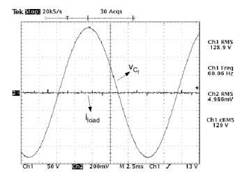
Fig. 13. No-load inverter output voltage.
