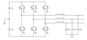
Fig. 6. Three-phase output inverter schematic diagram.
