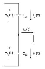
Fig. 5. DC bus capacitors voltage balance model.
