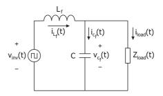
Fig. 7. Output inverter and LC filter schematic diagram.
