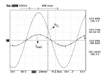
Fig. 14. Inverter output voltage and load current (10mV/A).
