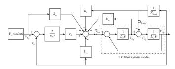
Fig. 8. Closed loop inverter output voltage control system.
