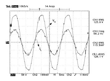
Fig. 11. Mains voltage (1:1 transformer) and line current (10mV/A).
