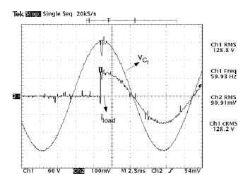
Fig. 15. Output voltage and load current (10mV/A).
