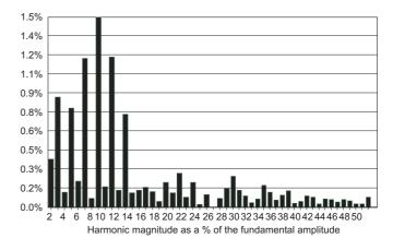
Fig. 17. Output voltage harmonic analysis.
