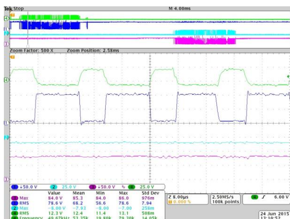
FIGURE 19. Voltage across Buck EI 2 switch (S3), in blue, and respective control signals, in green.
