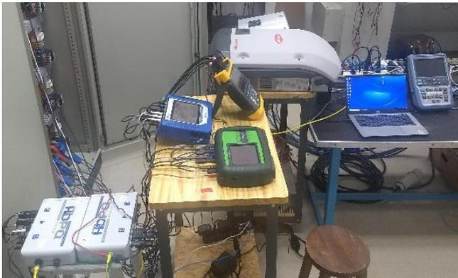
FIGURE 4. The experimental microgrid's measurement setup shows the PQAs, inverters, and additional instrumentation.
